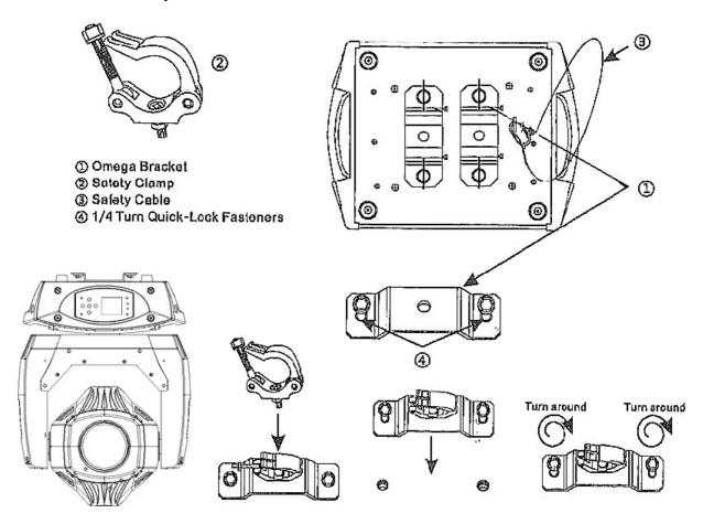
Regardless of the rigging option you choose for your 200W LED spot, always be sure to secure your fixture with a safety cable. The fixture provides a built-in rigging point for a safety cable on the hanging bracket as illustrated above. Be sure to only use the designated rigging point for the safety cable and never secure a safety cable to a carrying handle.
